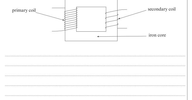
(b) A transformer is used to modify the mains power supply voltage in order to run a light bulb which is rated 50 W at 12 V.
